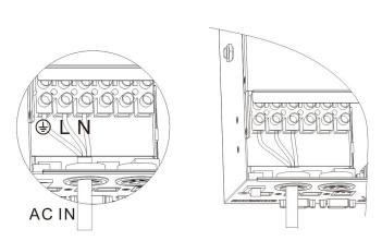
Correctly connect AC output wire in accordance with cable sequence and terminal position shown in the figure below. Please connect the ground wire at first, and then live wire and null wire. The ground wire is connected to the ground screw hold through Oshaped terminal.
