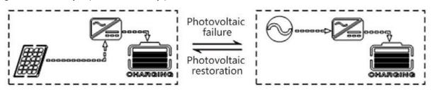
**2. Mains supply priority:** mains supply is to charge the battery preferentially and the photovoltaic charge can be started only when the mains supply is valid.
