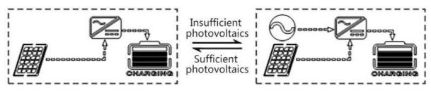
**4.Only solar:** only photovoltaic charge is used, no mains supply is started. This way can save the energy at most. The electric energies of battery are all from solar energy. This way is suitable for areas with good light condition.
