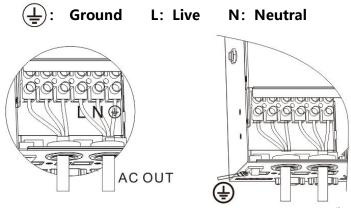
Note: use thick ground cable as far as possible (with cable section not less than 4mm<sup>2</sup>), place the ground point to be close to the all-in-one machine as far as possible and choose shorter ground wire to the greatest extent Wiring method of PV input:
